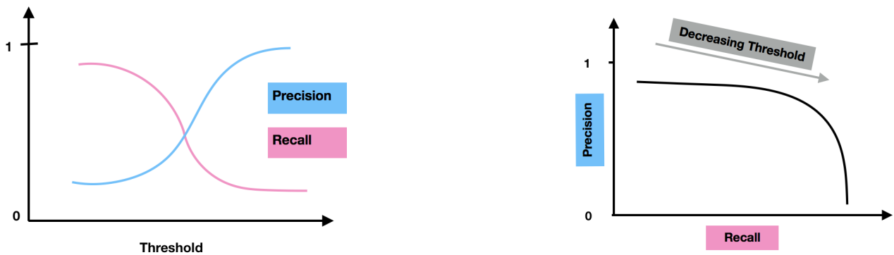
Figure 2.10: Illustration of how precision and recall individually vary with classifier's threshold. We can even vary Recall by implicitly adjusting the threshold to get various values of Precision as shown on the right.
