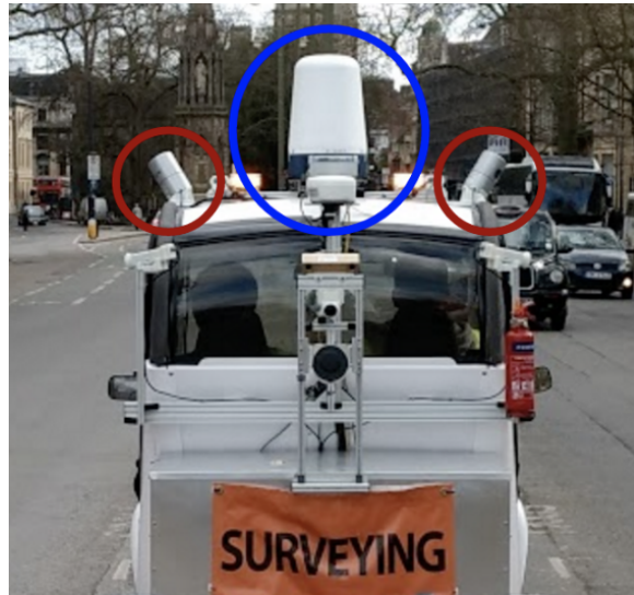
(b) RADAR sensor was mounted on the GEM surveying vehicle and the data used by us was captured by the ORI. Blue circle shows the radar and red shows two laser sensors[27].
