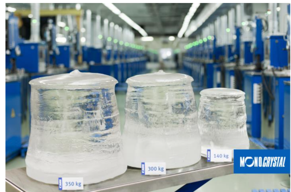
(b) Three large single crystal synthetic sapphire blocks made using the Kyropoulos process [61] .
